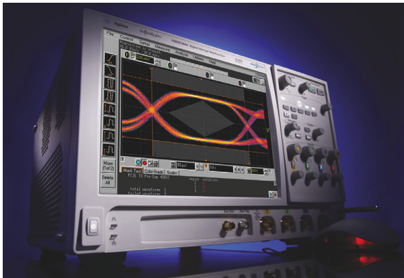
Infiniium 90000A oscilloscopes allow both bandwidth and memory upgrades. Any instrument is upgradable to the series maximum—13-GHz bandwidth and an industry-leading 1G-sample/channel acquisition-memory depth. Both figures apply to each channel, even with all channels active.
