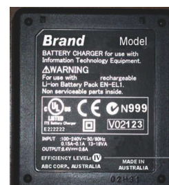
Figure 1 Although the Energy Star label on major appliances has a flashy Energy Star-compliance logo, the label on external power supplies is much smaller. Space constraints generally limit the designation to either III or IV, with III being the current spec, and IV indicating the tighter Version 2.0 proposed for 2008.
